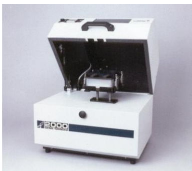
Figure 1. 2000 Geno/Grinder High-Throughput Tissue Homogenizer
